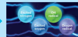
The electrons collide and combine with nitrogen and oxygen in the air to form four kinds of decomposing elements with decomposition power.
